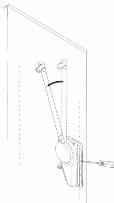
Attach the hanger-support pipe and use the lever positioned at the back to regulate the required power.
