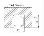
Size of the sink for assembling the quick release base on the door.
