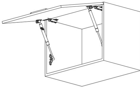
Assemble L Bracket & fix Bracket by using lock nut.
